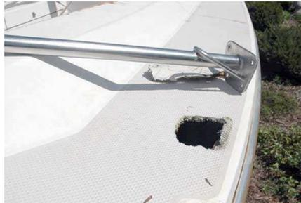
Stanchions are not meant to take the weight of snow and ice that can accumulate on a cover. And, as this photo shows, neither are the decks. This stanchion drove right through the deck on this 26-foot sailboat when the ice overloaded the stanchion and the deck beneath it. If you decide to cover the boat, do yourself — and your boat — a favor, and build a proper frame.
