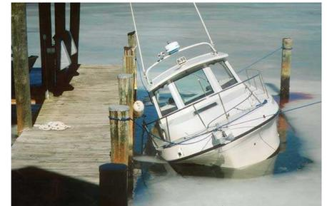
Snow accumulating in the cockpit can put above-waterline fittings below the waterline, with the inevitable result
