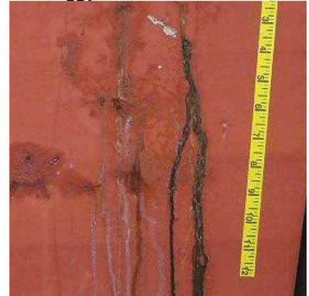
When you haul your boat for the fall and you notice that the rudder is dripping water a few days after it has been on the hard, or a keel has a blister that develops in the warm sunshine and recedes at night, the chances are you have water trapped in the rudder or the keel. If you leave it that way through the winter, it will freeze, and may damage the
