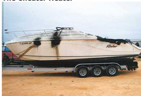
Our claim files show that "winterizing" a boat by leaving a heater running onboard is just not a good idea. First, your engine is least likely to be protected when it most needs it — in a big storm when the temperature plummets and the power goes out. Second, every winter we see fires from heaters,
