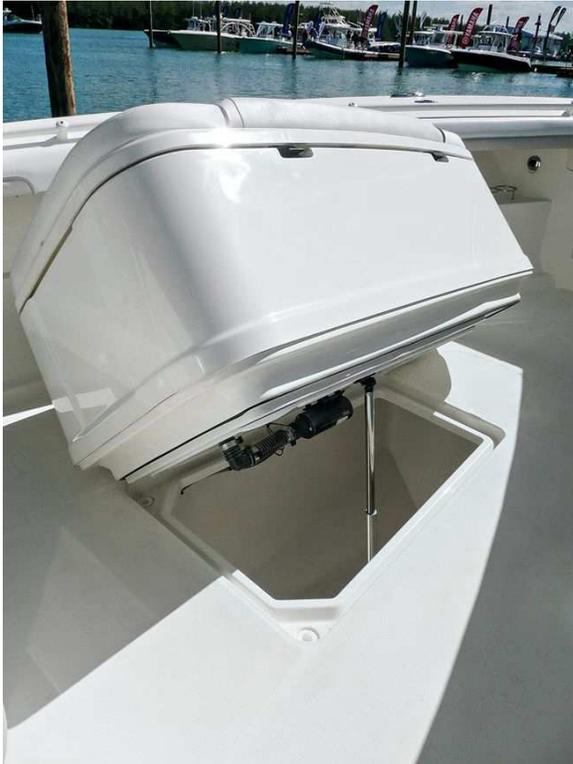
A box raises on a ram to access gear stowage underneath.
